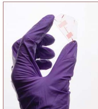
*A microfluidic chip. Microfluidics is the science of manipulating fluids on the micron scale, a unit of measurement much narrower than the diameter of a human hair.*
