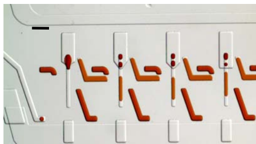
SI Figure 6. Microphotograph of an experimental test of different shapes at the junction of the capillary and receiving channel. The surface was treated with dichlorodimethyl silane to provide low contact angle hysteresis; the oil used was tetradecane. The capillary had depth 50\ \mu\text{m} , while the channel had depth of 78\ \mu\text{m} . The chip was slipped twice, increasing the overlap between the capillary and the channel each time, before the photo was acquired. The three right-hand channel geometries, which had angled and rectangular junctions, each caused the droplet to break after both slips. The left-most channel geometry, a gradual “fluted” expansion in width, minimized break-up of droplets and allowed the entire droplet to flow from the capillary into the channel. Scale bar is 1mm.
