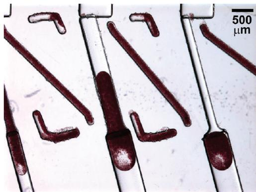
**Figure 8.** Spontaneous, capillary-pressure driven flow of whole human blood on an FEP-dipped SlipChip. Microphotograph shows droplets of citrated whole blood, 10 s after initiation of flow. The droplet on the right already finished flowing, while the flow of the left and center droplets was still in progress when the photo was taken. The carrier fluid was FC40 + 1 mg/mL RfOEG.
