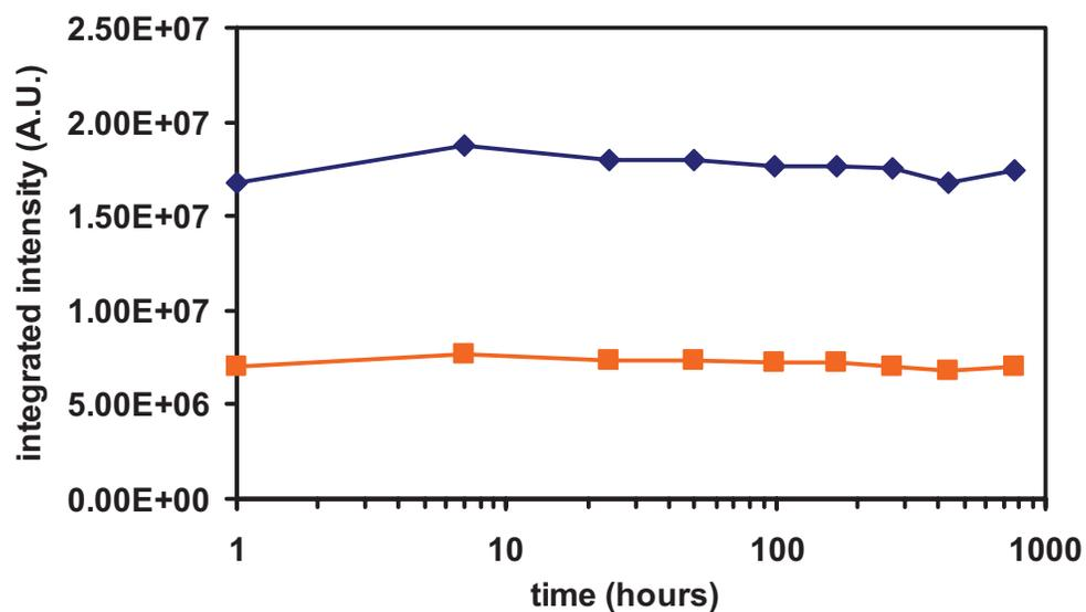
**Fig. S1.** Alexa-488 was used to characterize long term storage of reagent solutions in the SlipChip. Tracking the intensity (A.U.) of 2 individual wells over time indicated that the solutions in the wells were stable over 750 hours. In this experiment, the wells were covered by a silanized glass slide (500  $\mu\text{m}$  thick), and the whole chip was immersed in FC-70 for storage in the dark.
