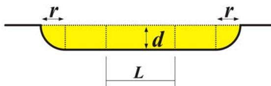
**Figure S2:** A schematic of an etched well illustrates the parameters used to calculate the volume of an etched well. The original pattern before etching is shaded and the etched area is shown in yellow.  $W_1$  and  $L$  are the original well width and length, respectively.  $W_2$  is the width of the etched well,  $r$  is the expanding distance (assumed to be the same in all directions), and  $d$  is the well depth. A) The top view of the etched well. B) The side view of the etched well.
