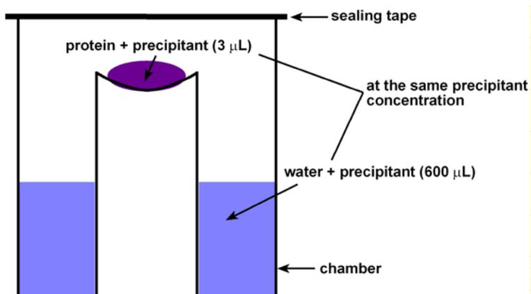
**Figure S3:** A schematic of the setup of the microbatch method used to scale up crystallization of proteins. The concentration of precipitant in the 600  $\mu\text{L}$  reservoir was the same as the concentration of precipitant in the 3  $\mu\text{L}$  well.
