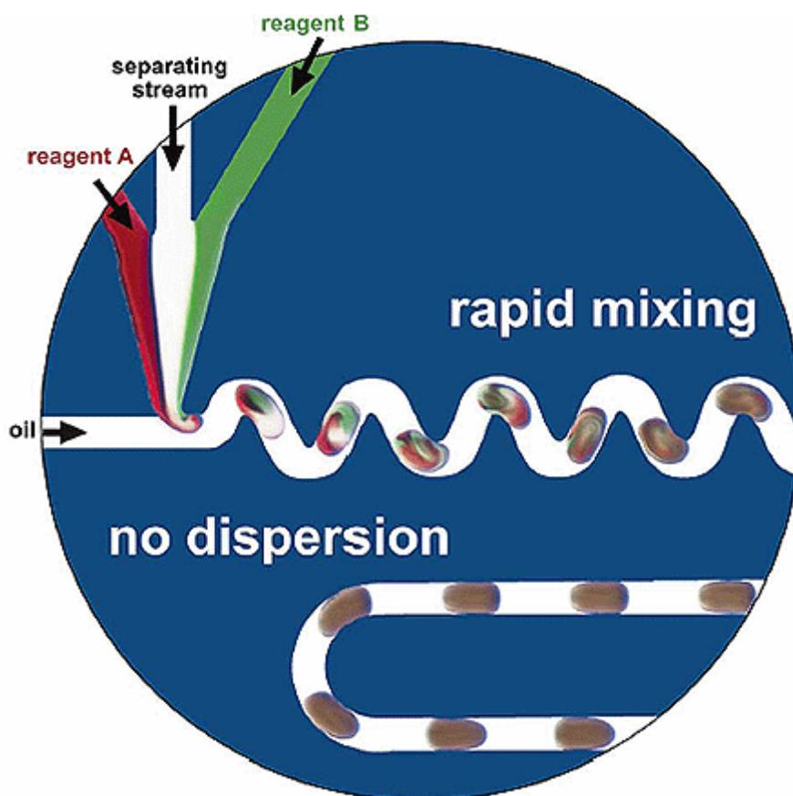
Aqueous droplets of 250 pL formed in a microfluidic channel in a continuous flow of a water-immiscible fluid act as microreactors that mix the reagents rapidly and transport them with no dispersion. These Droplets may also be used to control chemical reaction networks on millisecond time scale.
