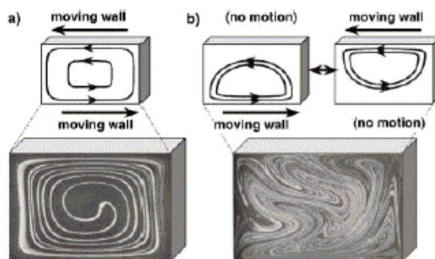
**Figure 3.** Mixing by steady (a) and time-periodic (b) flows in flow cavities. a, b) Top: Schematic illustration of the flow cavity. The vertical walls are stationary and the horizontal walls move as shown. Bottom: Images (reprinted with permission of Cambridge University Press from ref. [21]) that illustrate the flow patterns. For details, see text.
