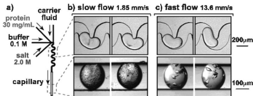
**Fig. 4** A schematic of the microfluidic plug reactor. (b) At low flow velocities precipitation occurs and microcrystals grow. (c) At high flow velocities no precipitation occurs and large crystals grow. (Adapted with permission. Copyright 2005, The American Chemical Society.)
