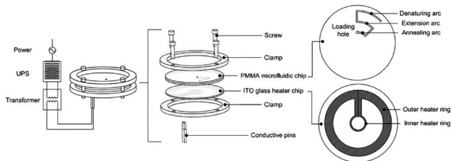
**Fig. 1** Microfluidic PCR reactor. The microfluidic and heater chips are clamped together. All components other than the glass chip and the conductive pins are made of plastic. The heater chip is fabricated from ITO-coated glass. The shaded area denotes the energized strips used for heating. The microfluidic chip is fabricated from PMMA.
