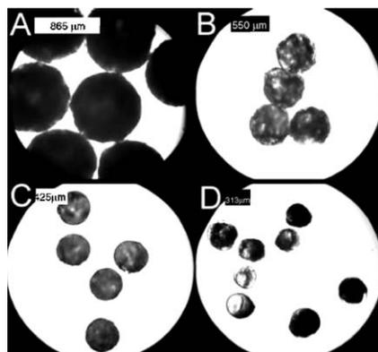
**Fig. 3** Light microscope images of capsules in water formed with constant organic flow rate ( $0.141 \text{ mL min}^{-1}$ ) and increasing aqueous flow rate: (A)  $2.00 \text{ mL min}^{-1}$ ; (B)  $11.0 \text{ mL min}^{-1}$ ; (C)  $13 \text{ mL min}^{-1}$ ; (D)  $25 \text{ mL min}^{-1}$ . (Adapted with permission. Copyright 2005, The American Chemical Society.)
