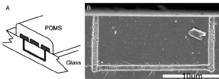
**Fig. 6** (a) Schematic of 'nanojumper' that joins two streams separated by a middle stream without mixing. (b) SEM of a cross section of the nanojumper. (Adapted with permission. Copyright 2005, The American Chemical Society.)
