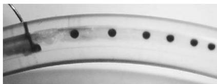
**Fig. 2** Photograph of fluidic device including needle and dye-filled organic droplets dispersed in the continuous aqueous phase. (Adapted with permission. Copyright 2005, The American Chemical Society.)
