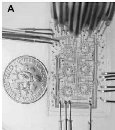
**Fig. 5** Optical micrograph of six microchemostats integrated on a single planar chip. (Adapted with permission. Copyright 2005, American Association for the Advancement of Science).
