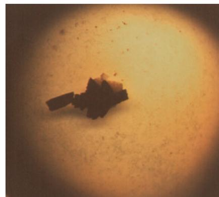
Light microscopy image of  $\alpha$ -crystacyanin from lobster shell, grown on bioactive gel-glass nucleant particles. Reprinted from ref. 3 with permission. Copyright 2006 National Academy of Sciences, USA.
