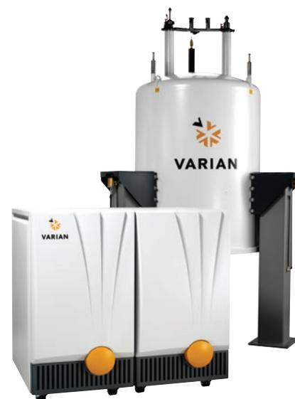
The Varian NMR System can be equipped with probes designed for increased sensitivity in high-salt biological solutions. (Courtesy of Varian, Inc.)
