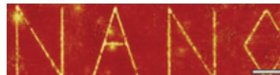
An AFM image of features etched onto a photoresist by evanescent waves focused by a silver superlens. Scale bar = 2  $\mu\text{m}$ . (Adapted with permission. Copyright 2005 American Association for the Advancement of Science.)
