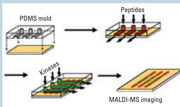
A schematic of a microfluidic peptide array.
