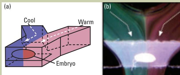
(a) A schematic of a fruit fly embryo developing inside a PDMS microfluidic device. (b) Thermo-chromic liquid crystals show a temperature step inside a microfluidic device—the green stream is 21 °C, and the red stream is 24 °C. (Adapted with permission. Copyright 2005 Nature Publishing Group.)
