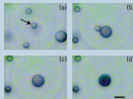
(a–d) A droplet containing the enzyme HRP (shown by arrow) is optically moved and fused to a droplet containing HRP's substrates. The chemical reaction is monitored by a color change. Scale bar = 250  $\mu\text{m}$ .
