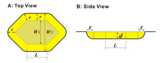
**Figure S2:** A schematic of an etched well illustrates the parameters used to calculate the volume of an etched well. The original pattern before etching is shaded and the etched area is shown in yellow.  $W_1$  and L are the original well width and length, respectively.  $W_2$  is the width of the etched well, r is the expanding distance (assumed to be the same in all directions), and d is the well depth. A) The top view of the etched well. B) The side view of the etched well.
