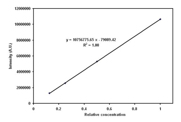
**Fig. S2** Alexa–488 was used to quantify the mixing ratio in the SlipChip. A dilution curve (3 data sets) with 4 points (1/8, 1/4, 1/2, and 1 times the original solution) was plotted to confirm the linear relationship between intensity (A.U.) and concentration. In this experiment, 5 nL of each solution was deposited into the wells in the bottom plate of a SlipChip. The wells were then covered by the top plate of the SlipChip and the fluorescent intensity of each well was measured.
