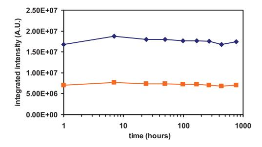
**Fig. S1.** Alexa–488 was used to characterize long term storage of reagent solutions in the SlipChip. Tracking the intensity (A.U.) of 2 individual wells over time indicated that the solutions in the wells were stable over 750 hours. In this experiment, the wells were covered by a silanized glass slide (500  $\mu$ m thick), and the whole chip was immersed in FC–70 for storage in the dark.
