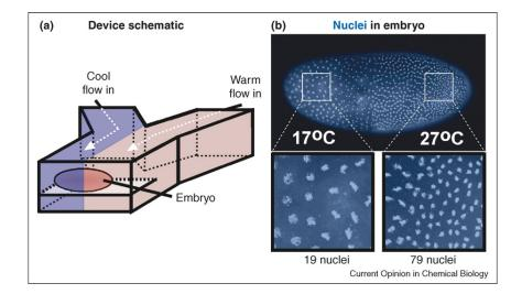
Microfluidic interface technology to control the development of a *Drosophila* embryo in space and time (adapted from Ref. [54]). (a) Schematic drawing of a temperature step around a live embryo in a microfluidic device. (b) As visualized by the difference in nuclear density in the two halves of the embryo, the difference in temperature affects the rate of development in each half of the embryo, with the cool half developing more slowly than the warm half.
