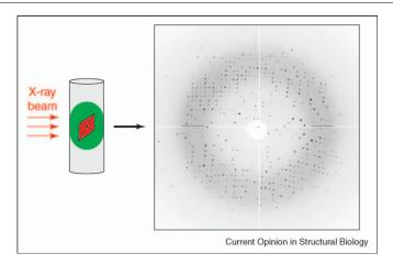
In situ diffraction of a thaumatin crystal at 1.8 Å resolution. A crystal was grown inside a plug in a capillary. The capillary was mounted on a goniometer and the crystal, while still in the plug, was subjected to the X-ray beam to obtain the diffraction pattern. The diffraction pattern is comparable to those obtained from crystals grown using conventional methods. The thaumatin crystal was ~100 × 100 µm and data were collected at Argonne National Laboratory's BioCARS beamline sector 14.
